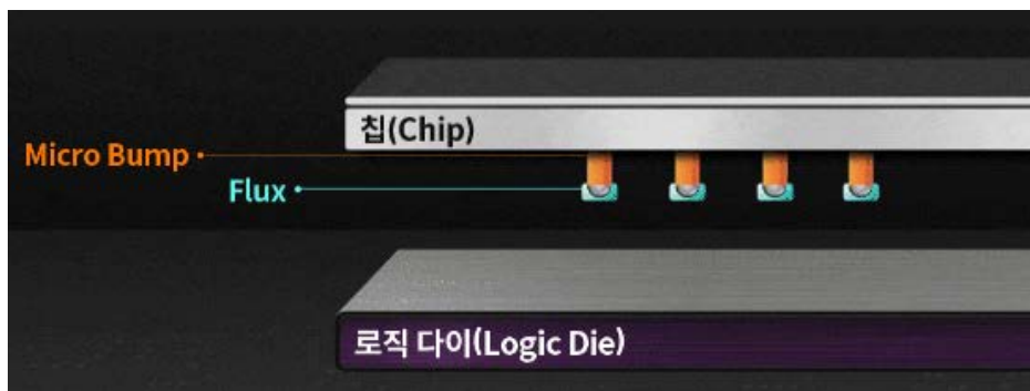
Fig. 63: (Advanced) MR-MUF Reflow 공정 내 Flux
